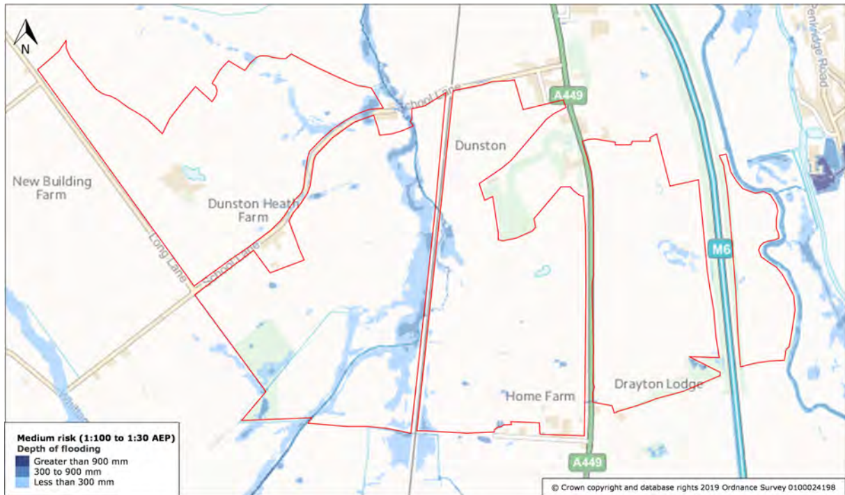
Figure7b: Risk of Flooding from Surface Water – Depth – Medium Risk
