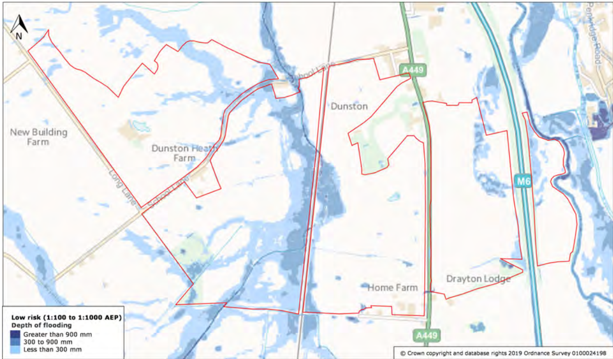
Figure 7c: Risk of Flooding from Surface Water – Depth – Low Risk (Source: https://flood-warning-information.service.gov.uk/long-term-flood-risk/map website)
