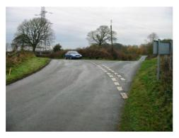
The position of the crossing is at the point where the two lanes meet which means that the road width and therefore length of the culvert would be greater than the normal road width. This would however assist in the construction of the culvert as one arm of the junction could be closed and half of the structure built with the closed section of road serving as site accommodation and access. The second half of the structure could be built by switching to a closure of the other arm of the junction.
